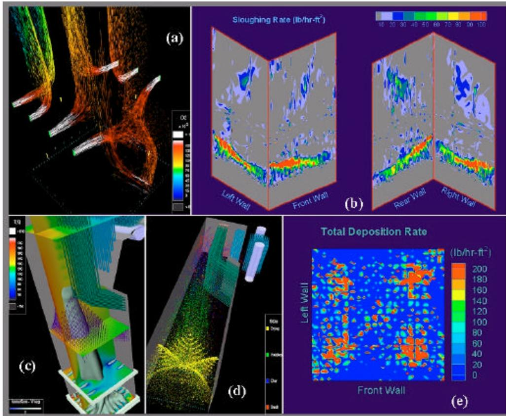
Figure 5: Example of boiler analysis: (a) tertiary air interaction, (b) wall sloughing rates, (c) air split ratios analysis and air core formation, (d) black liquor fuel states, and (e) unburned liquor deposition rate onto bed
