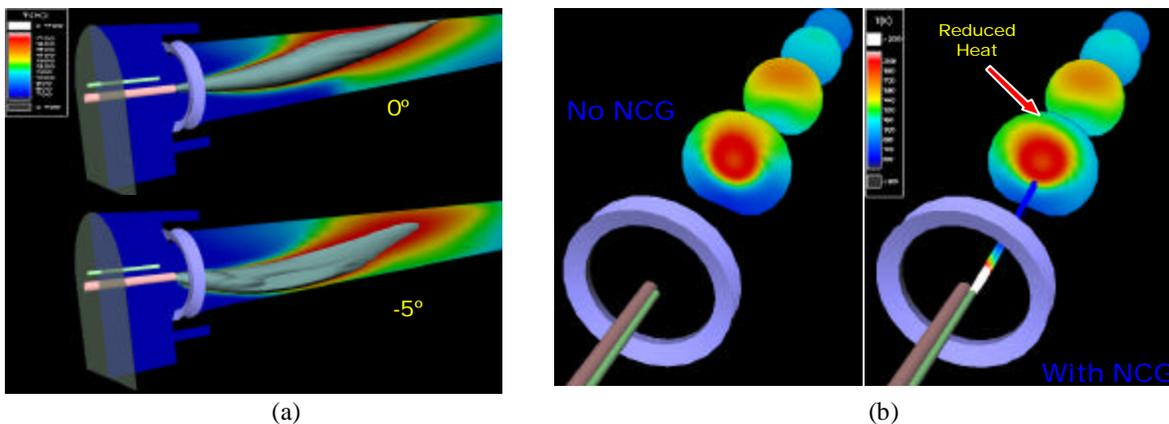
Figure 6: Optimization of the burner angle and the NCG injection location
