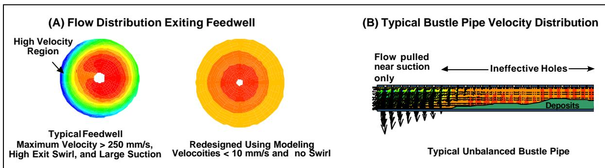
Figure 3: Application of CFD to a green liquor (a) feedwell, and (b) bustle pipe
