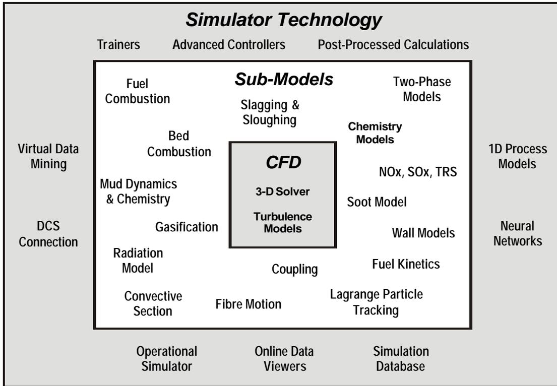
Figure 1: Advanced process modeling: CFD, sub-models, and simulator technology
