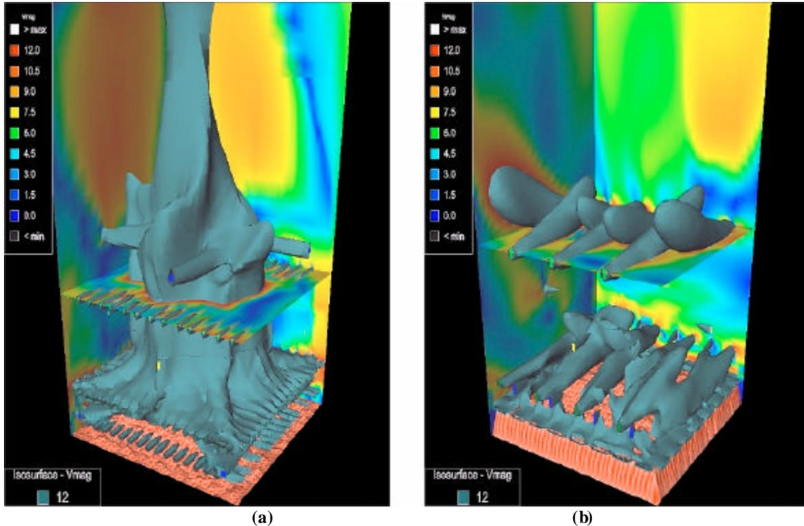
Figure 4: Traditional Versus Advanced Process Modeling Designs of a Recovery Boiler Air and Fuel Delivery System
